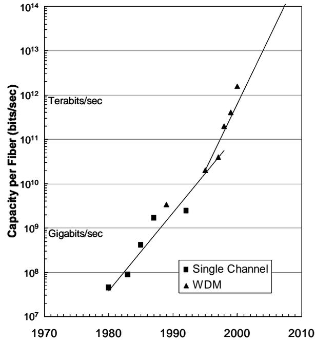
**Figure 7. Optical transmission capacity has grown exponentially for 20 years. Recent research indicates the theoretical capacity limit is about 100 terabits/second (10<sup>14</sup> bits/second).**
